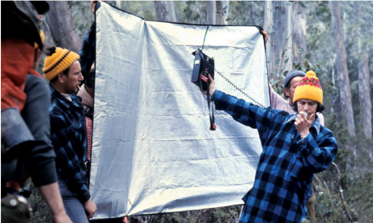
Unsuccessful experiments were conducted to see if a reflector (an aluminised groundsheet) would improve the range of the VHF set.
